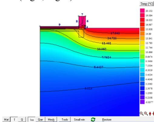
**Fig. 4** Isotherms of horizontal insulated floor in summer period.
