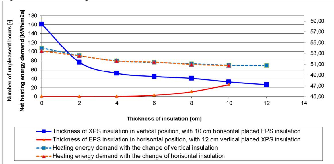
**Fig. 3** The number of unpleasant hours and the net energy demand of the whole building depending on the design of the floor at the first building.
