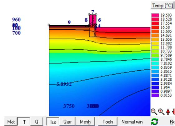
**Fig. 5** Isotherms of vertical insulated floor in summer period.
